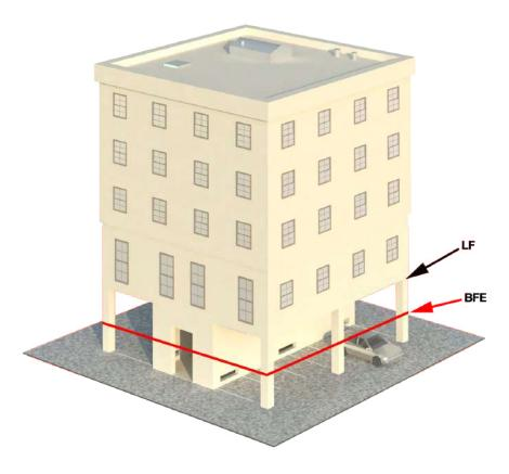
Figure 2-3. An apartment building with entrance, storage, and parking below BFE
