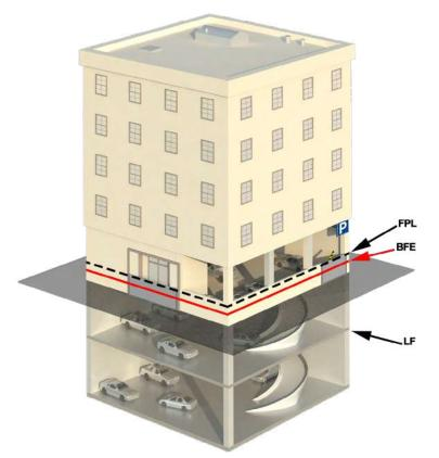
Figure 6-5. Illustration of Scenario 5 – Dry floodproofed below ground parking area
