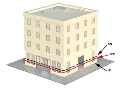
Figure 6-2. Illustration of Scenario 2 –Dry floodproofed ground level
