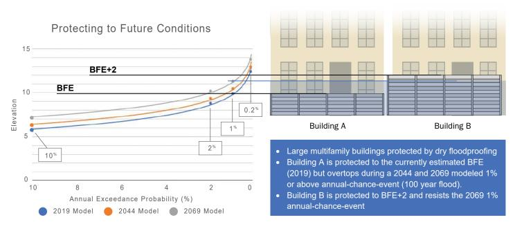
Figure 3-6. Value of freeboard to address future conditions; this example assumes 39 inches of flood level rise by 2100 and includes wave action.
