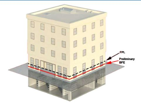
Figure 6-4. Illustration of Scenario 4 – Dry floodproofed basement areas for a building outside the SFHA
