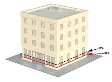
Figure 5-3. Example of dry floodproofed multi-family building (FPL must be at BFE for compliance with the minimum NFIP requirements and greater than BFE +1 ft for insurance credit)
