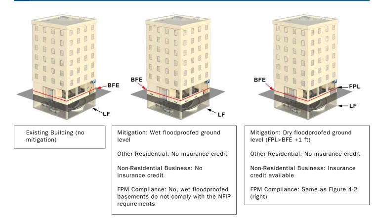
Figure 4-5. Image (left) shows the lowest floor of a multi-family building with pedestrian access and below grade parking access at ground level (no mitigation measures), image (center) shows the lowest floor with a noncompliant wet floodproofed enclosure, and image (right) shows the dry floodproofing of the ground floor, which is all non-residential
