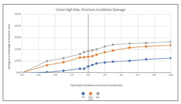
Figure 2-7. Depth damage function for a 10-story urban high-rise building (Source: USACE 2015)
