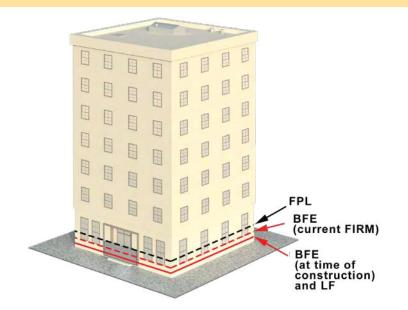
Figure 6-6. Illustration of Scenario 6 – Dry floodproofed ground level of legal non-conforming construction
