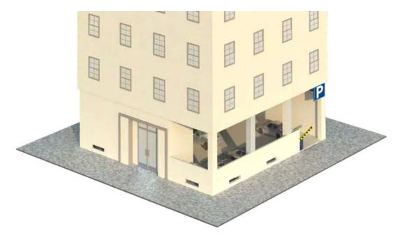
Figure 5-2. Example of a wet floodproofed multi-family building (note flood openings around the ground level of the building)
