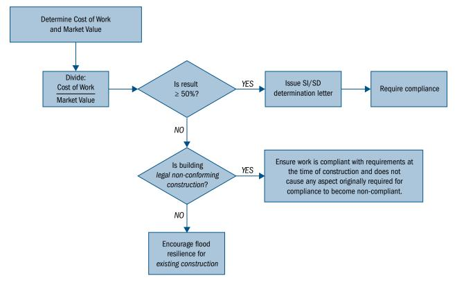
Figure 2-6. Overview of the SI/SD determination process
