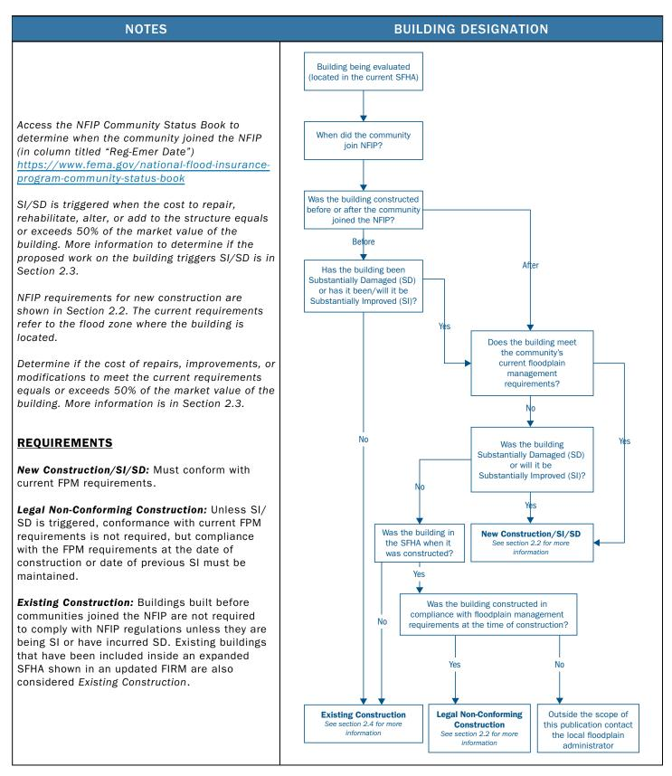
Figure 2-1. Determining the Building Designation
