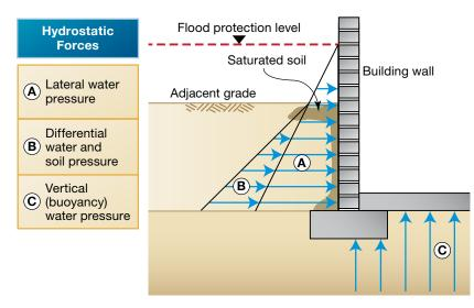
Figure 3-4. Hydrostatic loads
