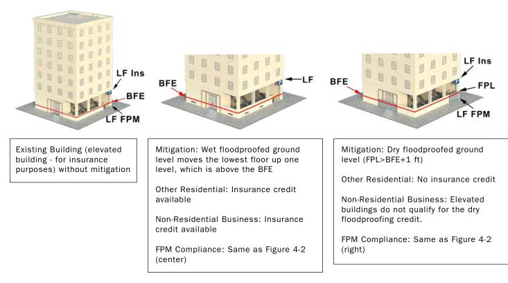
Figure 4-4. Image (left) shows the lowest floor of a multi-family building with parking and access at ground level (no mitigation measures), image (center) shows the lowest floor with a compliant wet floodproofed enclosure, and image (right) shows dry floodproofing of the ground floor, which is all non-residential
