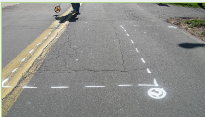
Typical survey paint markings
